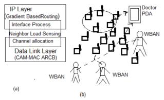
Figure 8. Adaptive routing solution: (a) cross-layered integrated solution and (b) routing around high-network load regions with different priority
