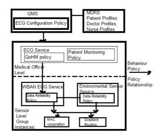
Figure 6.Overall Group Instance Policy Perspective identifying the relationship to both MAC and routing technologies
