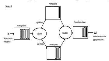
Figure 2. Packet Classification and Packet Scheduling at a Sensor
