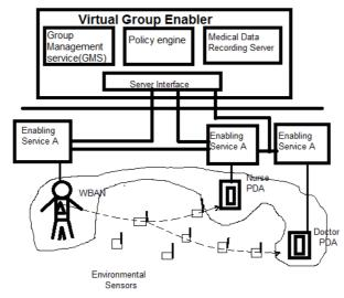
Figure 3. Overall Virtual Group Enabling Architecture
